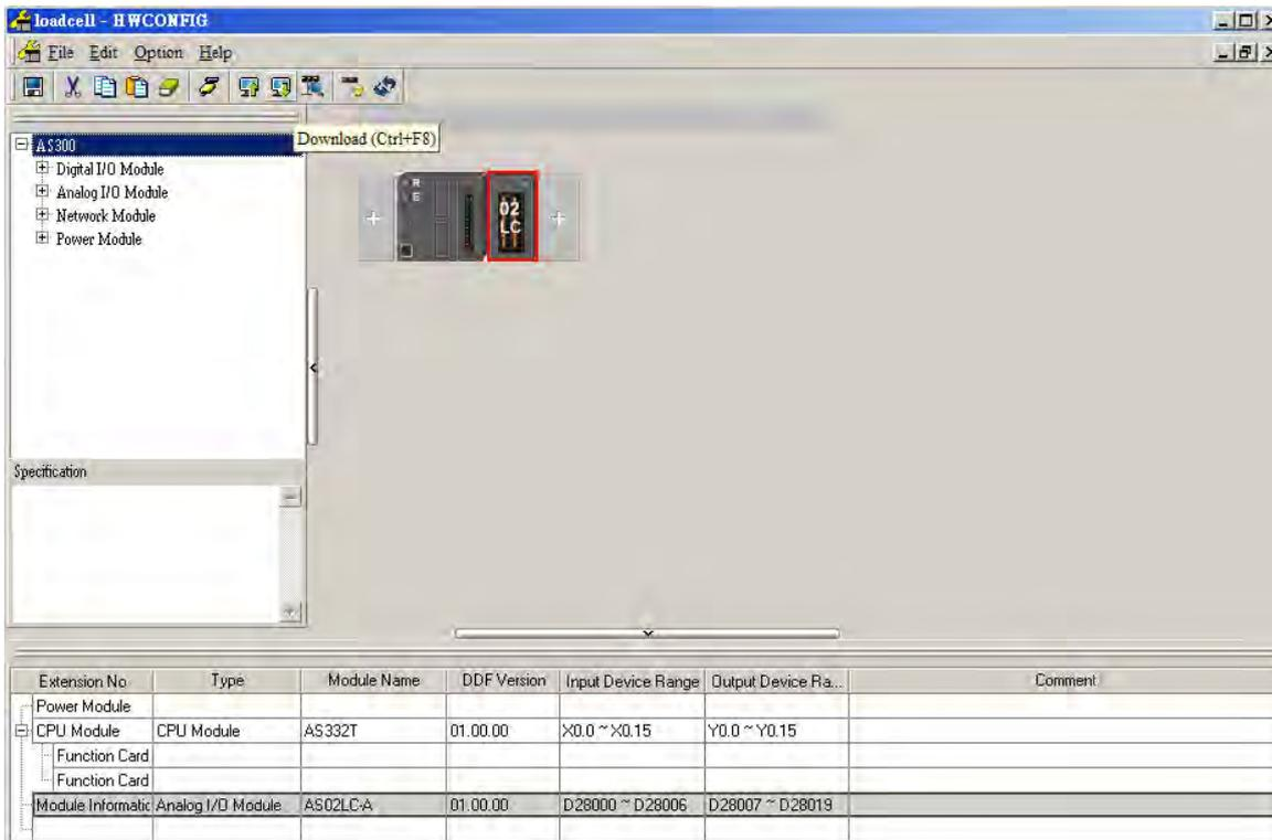
Step 4: Users can see the corresponding address for instruction is D28007 in the Normal Exchange Area.
