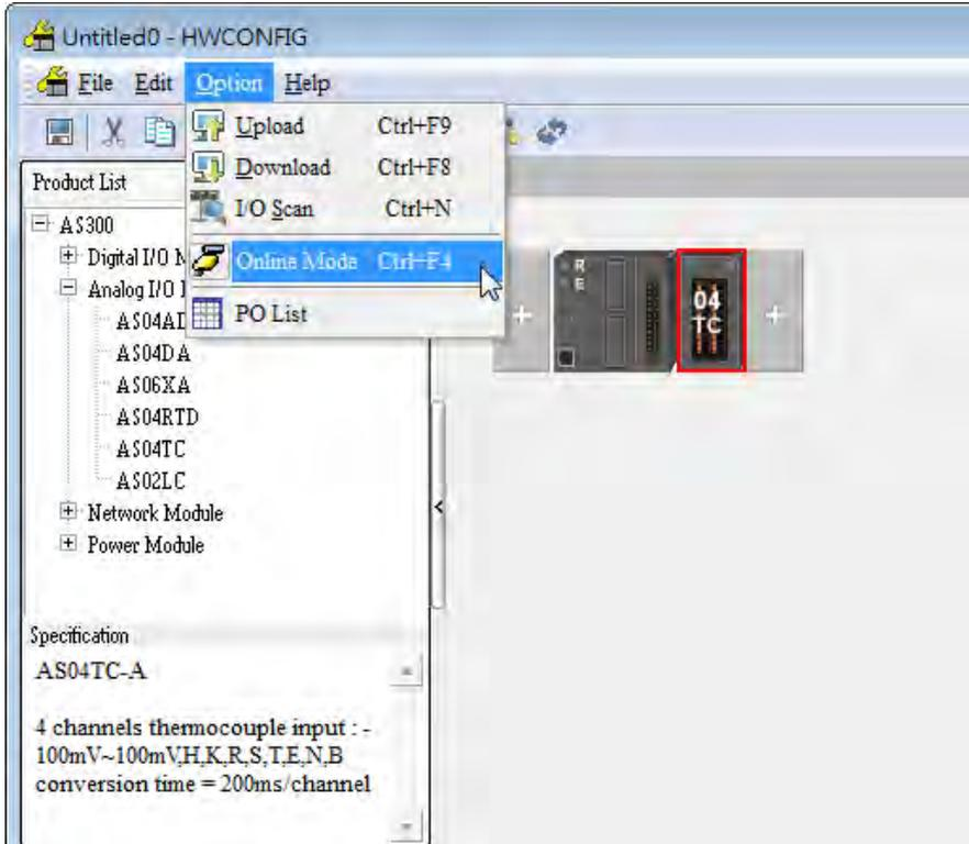
(2) Double-click the module to see the Device Setting page. The version of the firmware and that of the hardware are displayed.
