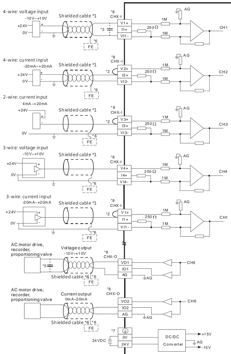
\*1. Please use shielded cables to isolate the analog input signal cable from other power cables.
