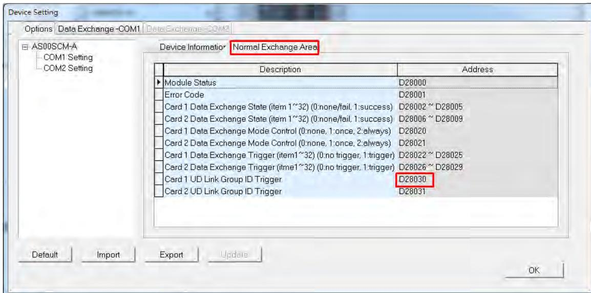
Users can use the monitor function in ISPSOft to see if the transmission works correctly.
