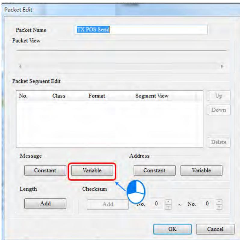
Input the data registers that contain the values you'd like to obtain. The example here uses D26100 and the obtained value length is 3 byte.
