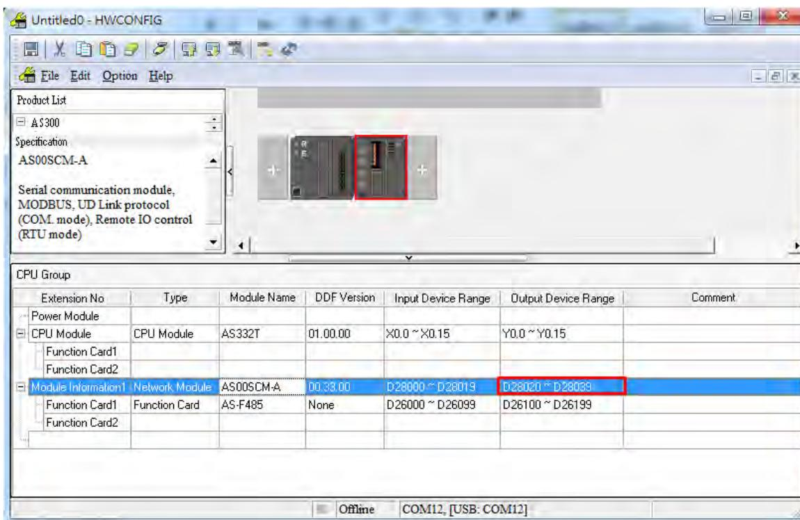
Double-click AS00SCM to open the device setting page. Users can see the Card 1 UD Link Group ID Trigger is in D28030. Write 1 into D28030 via ISPSOft to trigger and start data exchange.
