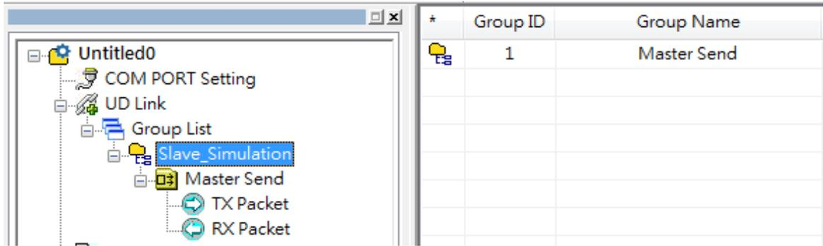
7) Edit the TX Packet and name it as TX POS Send. Double-click TX POS Send to open the Packet Edit window.
