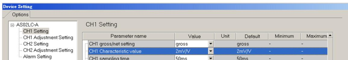
Step 2: Set up 2-point adjustment; when the sensor is loaded with a 10Kg weight, set up the value to 10.
