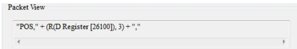
[yyy] is variables. Click Variables to edit. The value is obtained from the value in data register (D26100~D26199) via ISPSOft. The example here uses D26102: 16#3132 and D26103: 16#3300 and the value obtained is 123.
