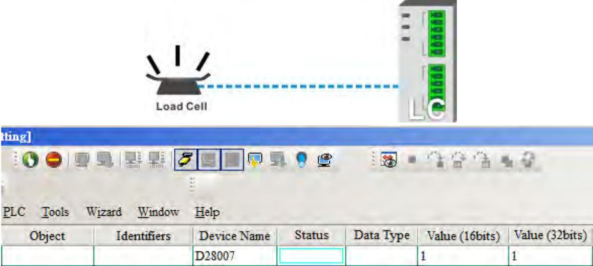
Step 7: Put a load on the load cell (adjustment point 2). For multi-point adjustment, repeat this step. This example uses a 1Kg.
