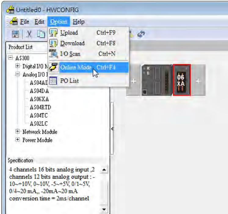
(2) Double-click the module to see the Device Setting page. The version of the firmware and that of the hardware are displayed.
