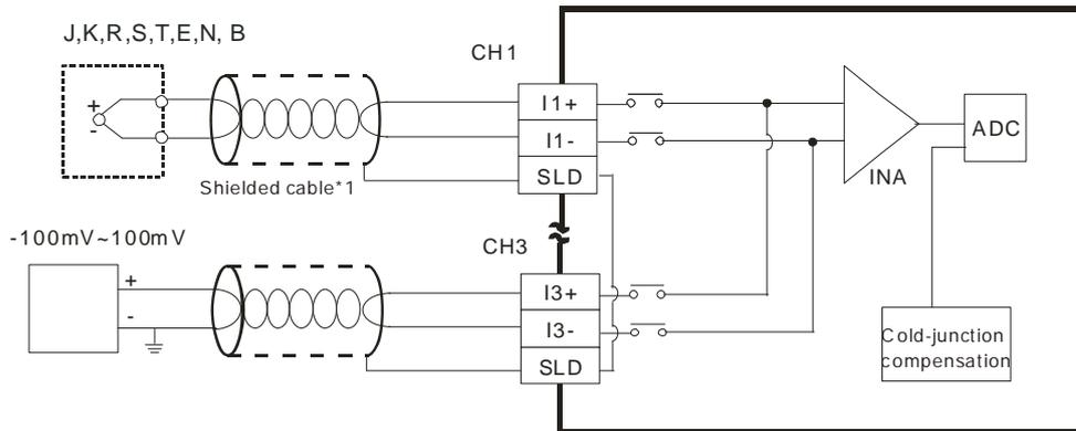
\*1. The cables or the shielded twisted pair cables for Type J, type K, type R, type S, type T, type E, type N and type B thermocouples are used, and should be kept separate from other power cables and cables which generate noise.
