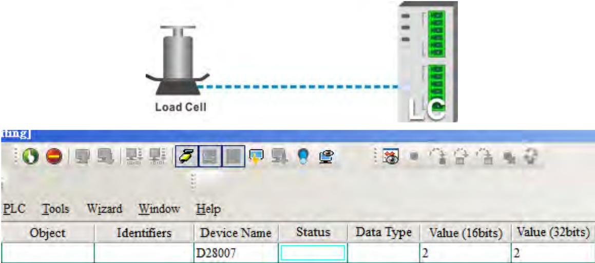
Step 8: Write the instruction of inactivating the weight calibration 99 into D28007 and the adjustment is done.
