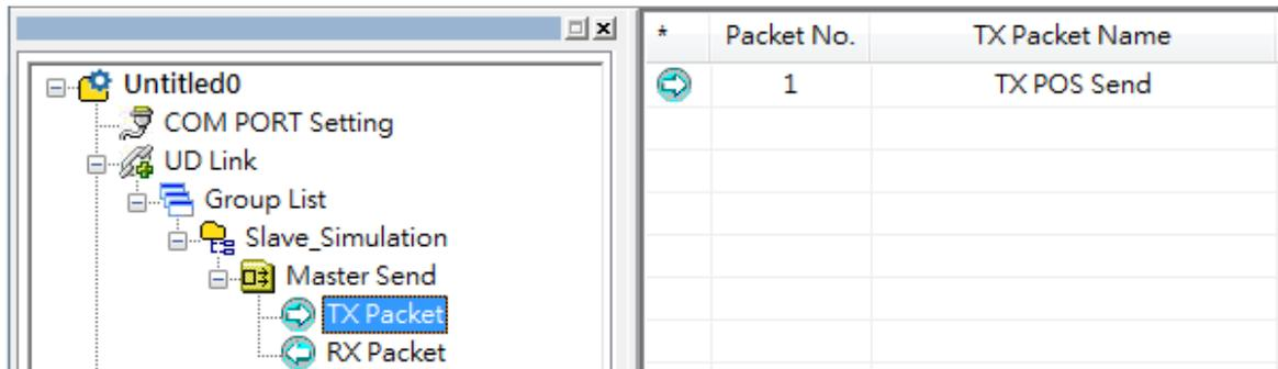
Edit the TX packet, "POS, xxx, yy" (the example below uses POS, 123, 123)
