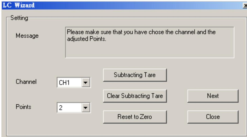
Step 6: Put no load on the load cell (adjustment point 1). And click "Next" to proceed.
