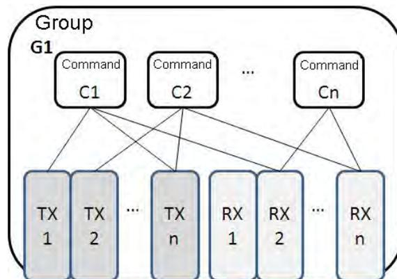
First, create TX packets and RX packets in a group. Then, set the sequence of sending/receiving the packets, and the number of times the packets are sent/received through commands. Finally, the sending/receiving of the packets in the group is triggered. Besides, if several different types of packets are required in a larger system, users can arrange several groups in sequence, and set the sequence of sending/receiving the packets in the groups.
