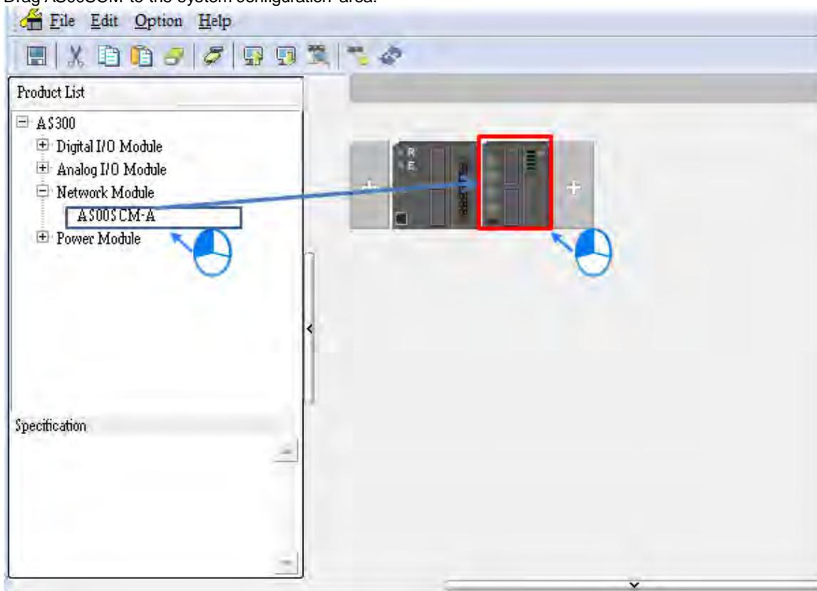
2) Double-click the SCM module to open the device setting for configurations.
