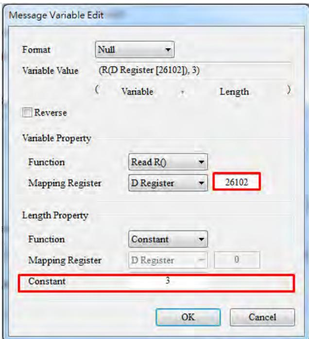
Input the data registers that contain the values you'd like to obtain. The example here uses D26102 and the obtained value length is 3 byte.
