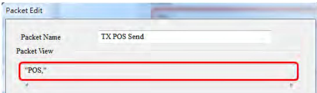
[xxx] is variables. Click Variables to edit. The value is obtained from the value in data register (D26100~D26199) via ISPSOft. The example here uses D26100: 16#3132 and D26101: 16#3300 and the value obtained is 123.
