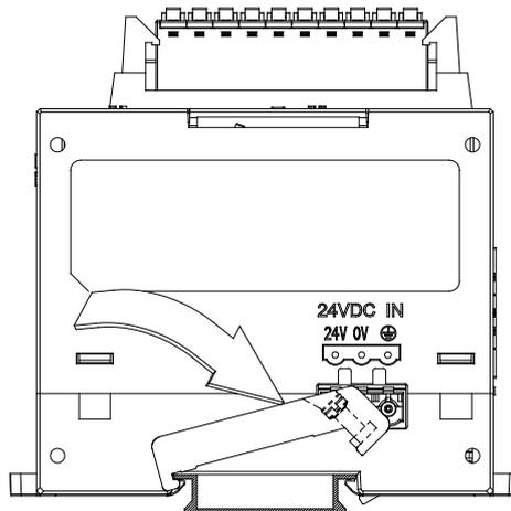
2. Use screws to secure the baffle.
