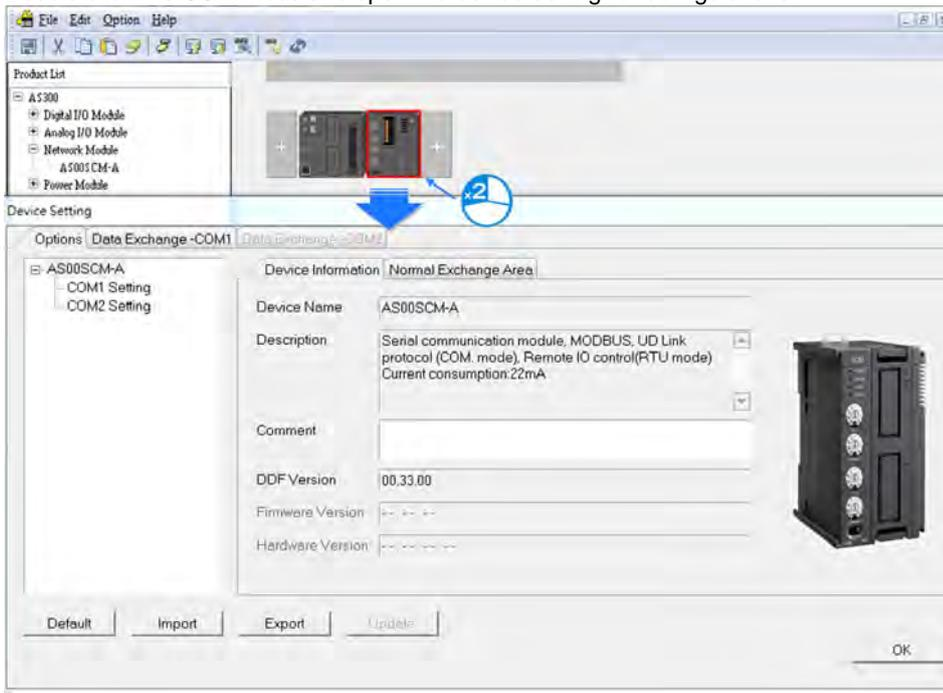
3) Select AS-F485 in the function card type for COM1. And its corresponding parameters will appear.
