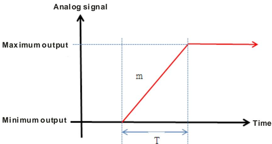
When the analog output signal changes, the value of the analog output will be updated according to the value set in the slope as the image shown below.
