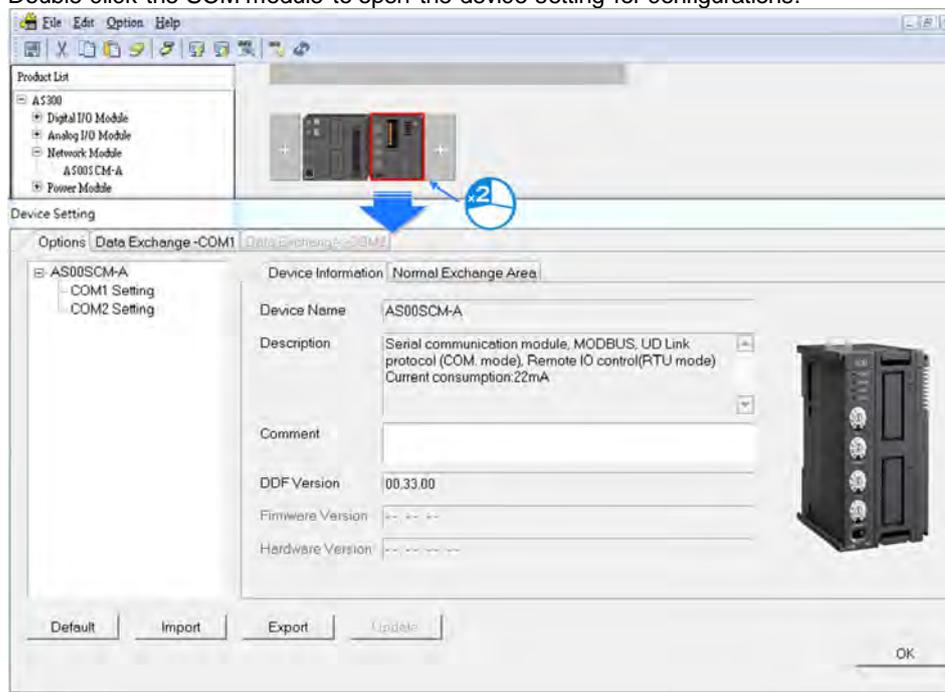
4) Set up the protocol for COM1 to be the same as the format of HMI in the Options page.
