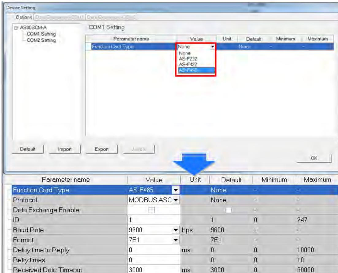
4) Select UD LINK in the protocol. Set up the baud rate and format. Click OK.
