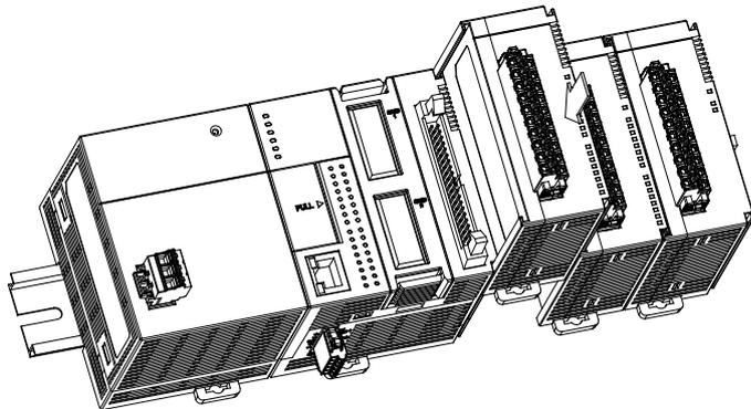
3. When the installation is done, secure the module with screws.
