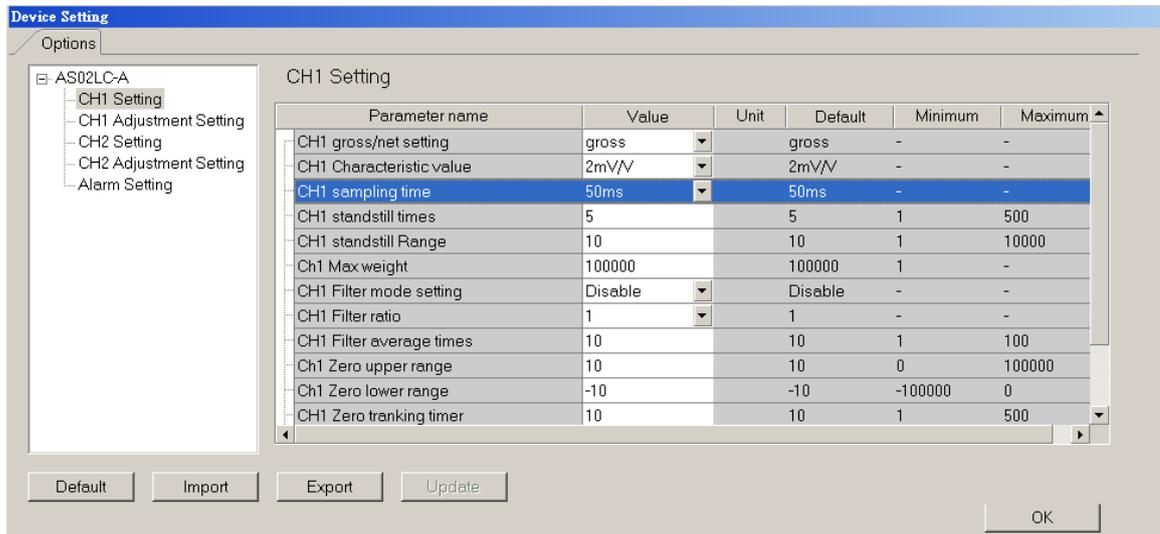
Step 2: Set up the number of adjustment and its corresponding value; the example is a 2-point adjustment, point 1 is 0 and the value for point 2 is 1000, corresponding to 1Kg.
