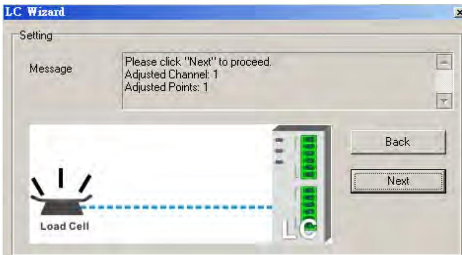
Step 7: Put a load on the load cell (adjustment point 2). For multi-point adjustment, repeat this step. This example uses a 1Kg.
