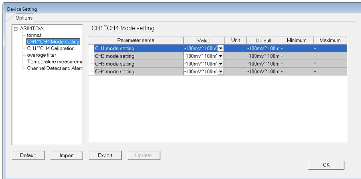
(5) Click **Download** on the toolbar to download the parameters. (The parameters can not be downloaded when the CPU module runs.)
